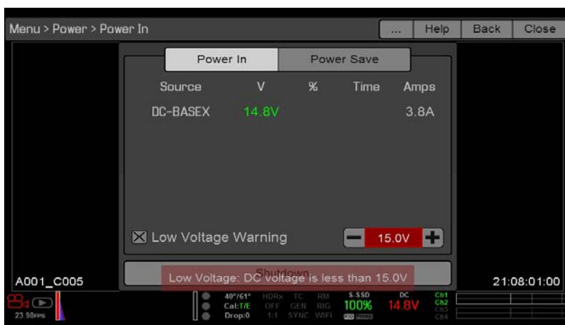
Figure: Low Voltage Warning
