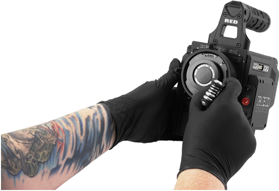
Figure: Remove the Lens Mount Screws
