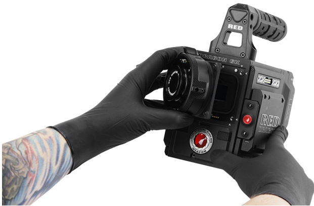
Figure: Align Lens Mount Pins
