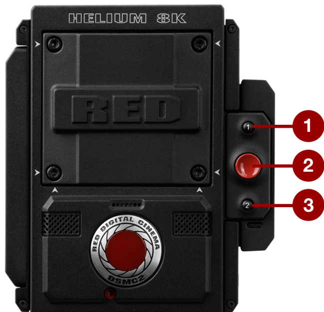
Figure: Media Bay Controls
