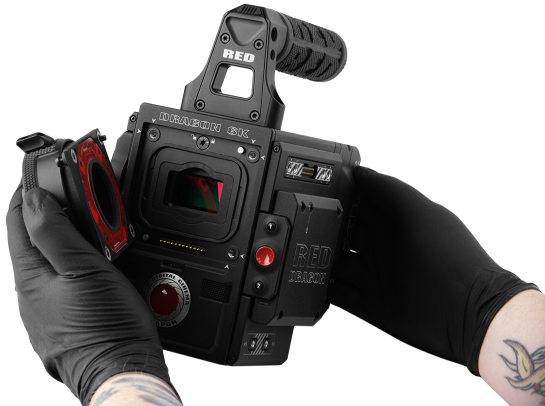
Figure: Remove the Lens Mount
