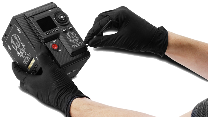
Figure: Reinstall the Side Module/Panel
