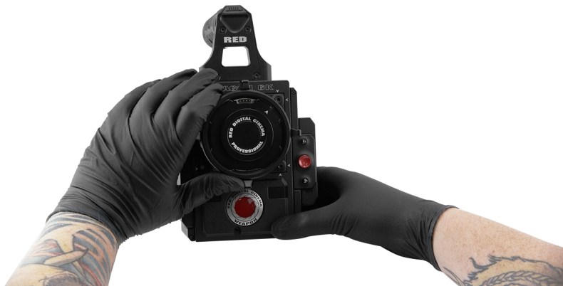
Figure: Turn Locking Ring Counter-Clockwise
